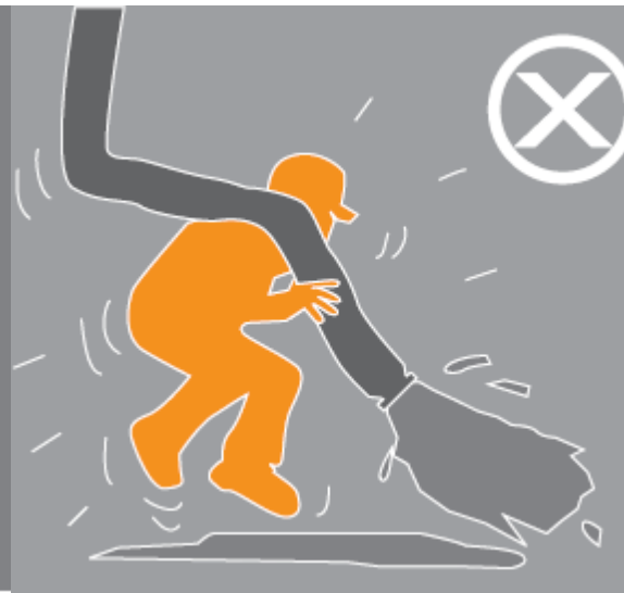
Figure 15: Let the boom do the work
